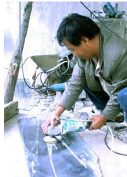
A stone painting undergoes a wax finish and polish of special organic and inorganic waxes
