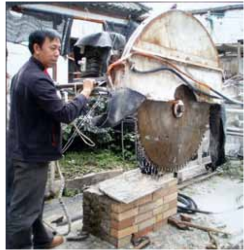
Giant saw slices through raw stone slabs; the cutter hoping to reveal a precious dream stone painting
